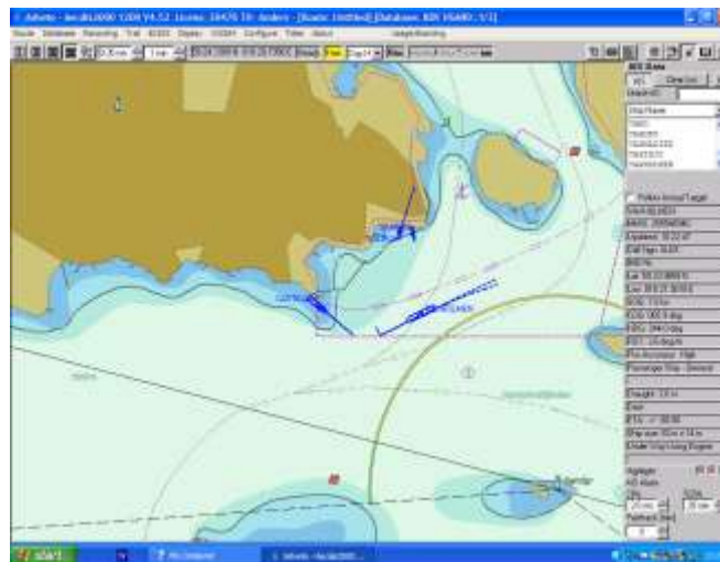
Figure 37 Example of how AIS is presented in the navigational software ADVETO AECDIS.
