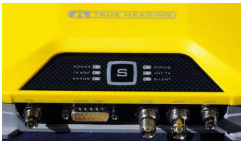
Figure 7 AIS-CTRX CARBON + connectors. From the left FME (Female) for FM radio (a 1,6 m prepared cable comes with delivery), 15 pole d-sub connection (Male) for data and DC power supply, TNC (Female) for GPS antenna, BNC (Female) for VHF antenna (a BNC to UHF adapter is provided if required). We do however recommend to use a BNC connector direct on the VHF antenna cable. Finally to the right a FME (Female) connector for the VHF radio (a 2 m prepared cable comes with delivery).
